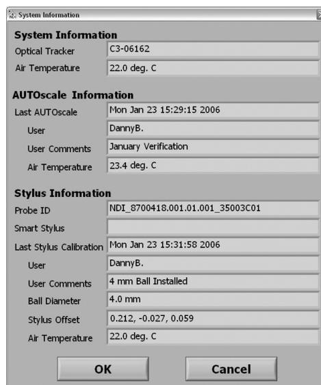
Figure 4-1 Example Stylus Calibration System Information Window
