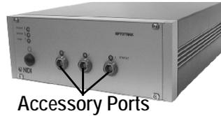
Figure 3-4 Wired Accessory Connections
